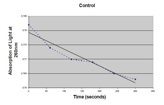
**Figure 5**: Hewlett Packard spectrophotometer readings of an aqueous solution of human placental DNA rewinding immediately following heat treatment in control conditions. Solid black line is computer generated best fit analysis used to calculate the slope (absorption/time) which is used as the rate of rewinding. The slope of this line is increased in the presence of cellular phone radiation.
