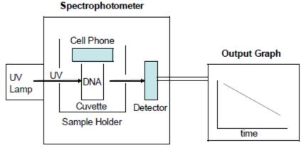
**Figure 3:** To measure rewinding, an aqueous sample of human DNA is placed in a cuvette inside a Hewlett Packard spectrophotometer which measures the absorption of UV light by the sample. Light absorption is measured every 10 seconds when the DNA is spontaneously rewinding. Note the position of the cellular phone whose radiated EM field influences the rewinding process of the DNA inside the cuvette underneath the cellular phone.
