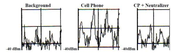
In this portion of the EM spectrum, it is clearly visible that the cell phone signal in the presence of the Neutralizer is quantitatively and qualitatively similar to that obtained from the
