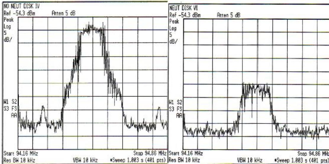
**Figure 7:** Typical spectrum analyzer traces centering at 94.16 MHz. Peak heights are related to the intensity of cellular phones radiation. Left trace is a recording from a normal cellular phone and the right trace is recorded from the same cellular phone with the shielding device attached.
