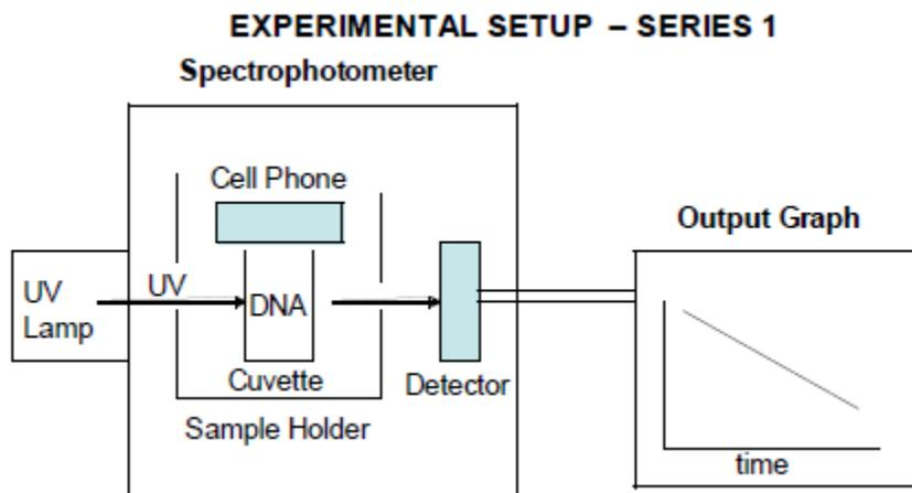
**Figure 3:** To measure rewinding, an aqueous sample of human DNA is placed in a cuvette inside a Hewlett Packard spectrophotometer which measures the absorption of UV light by the sample. Light absorption is measured every 10 seconds when the DNA is spontaneously rewinding. Note the position of the cellular phone whose radiated EM field influences the rewinding process of the DNA inside the cuvette underneath the cellular phone.
